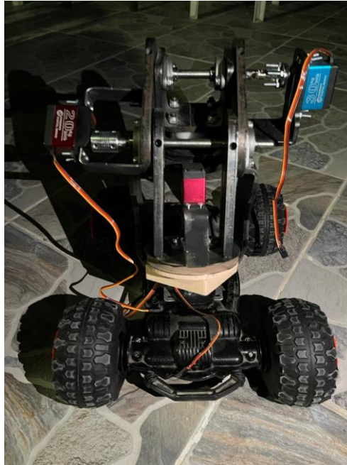
Figure 5.12 Compound mobile and serial robot arm
